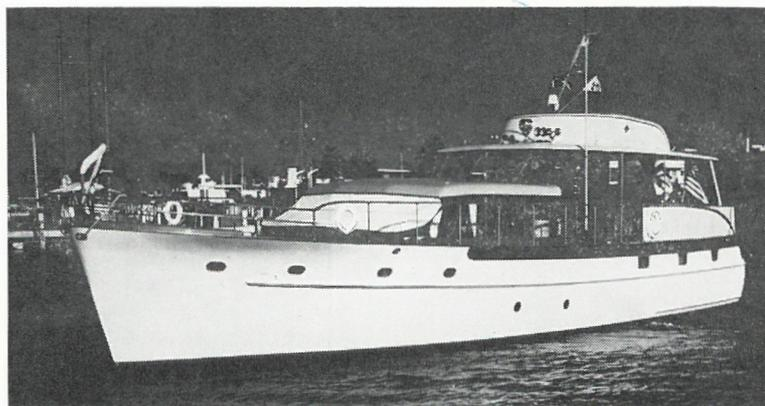
*A letter from H. J. Windolph describes the new flybridge added to MARA CAPRICE, Burger 60 delivered in the spring of 1958. "Note access to flybridge, sundeck is through a hatch in top deck and up an aluminum ladder. Installation is all aluminum with foam rubber seats and backrest and storage compartments. Removable aluminum ladder can be stowed in flybridge compartment. Total height is only 26 inches. For all other dimensions you are welcome to send anyone to take all dimensions.*
