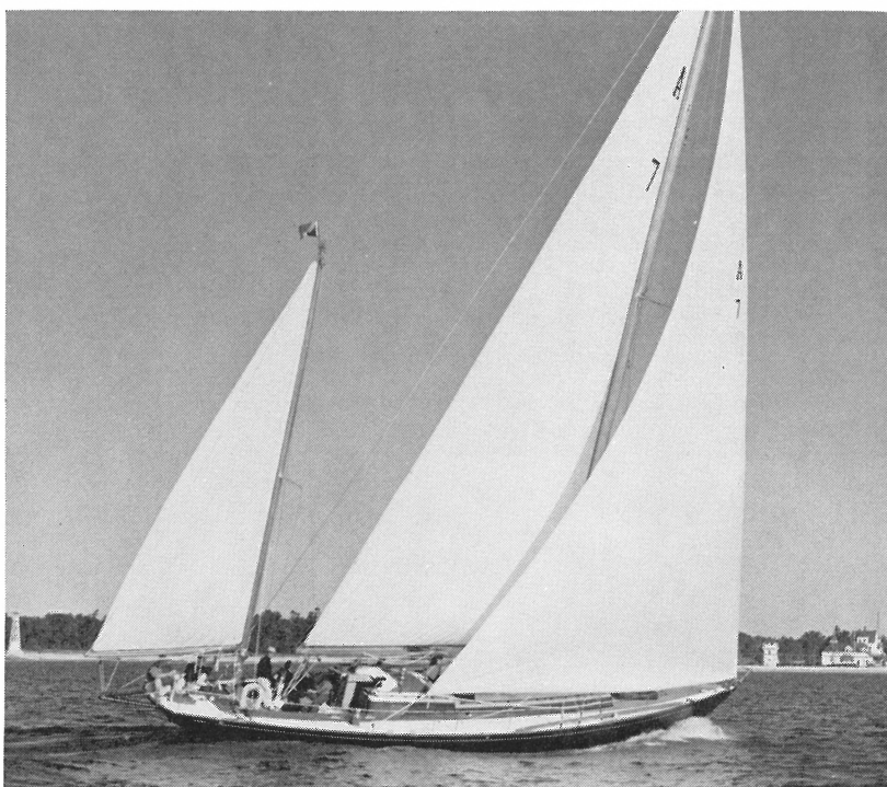
1954-1957 — Burger continued to lead . . . building the first all-welded aluminum hull in 1954. Then in 1957, DYNA (above) and ARIA were launched. They were the first and largest welded aluminum auxiliaries ever built in this country.
