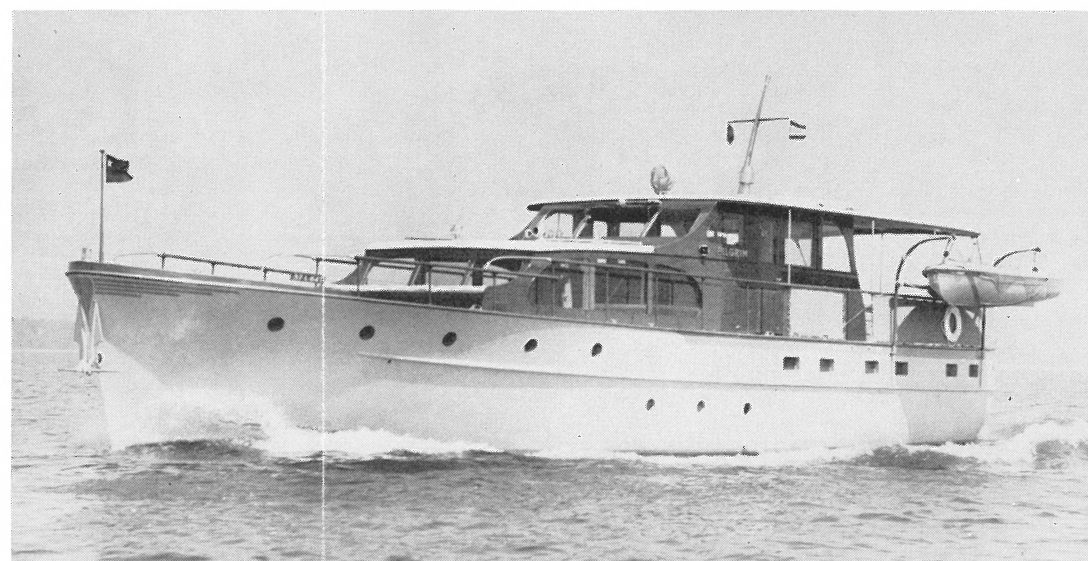
1941 — Burger continued to pioneer. First the steel hull . . . now Burger built the first flush deck cruiser. She was PILGRIM (above) a 65 footer launched in 1941. Her design was considered too "radical" by some builders of the period. However, the style of today's cruisers is ample evidence of Burger's leadership in yacht building.
