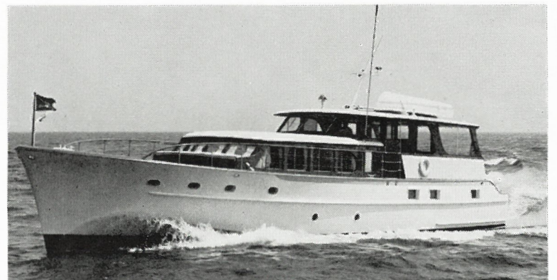
This 65' steel Burger for a Florida yachtsman is fully air conditioned and sports a fishing cockpit aft.
